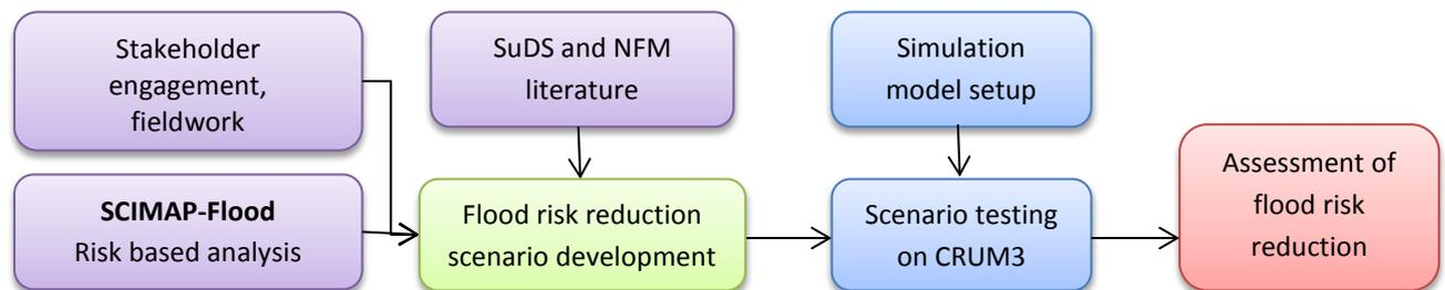
**SCIMAP-Flood:** risk mapping framework that enables analysis on a sub-field scale but across the catchment's extent using limited data inputs. It identifies key sources and flow routes through analysis of topography and land use, to give an understanding of the surface runoff regime at a catchment scale ([www.scimap.org.uk](http://www.scimap.org.uk))
